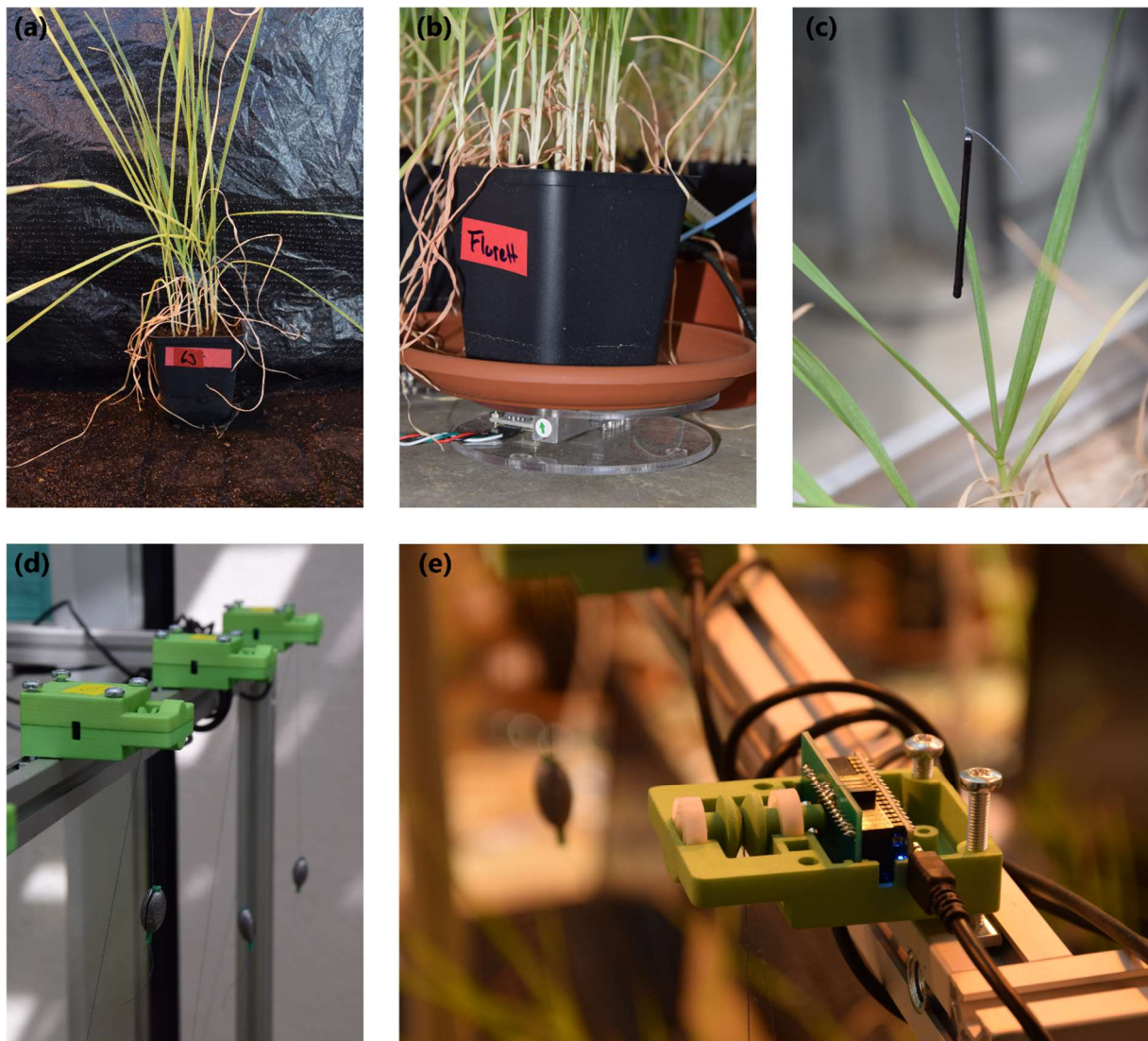
Fig. 8: Soil water deficit and leaf elongation rate tracking on phenotyping platform Monocot Envirotyping Unit. (a) 10 Wheat plants at leaf stage 6 ready to be measured on the phenotyping platform. (b) Pots are placed on a scale for a continuous measurement of soil water deficit. (c) Youngest leaf of one plant per pot is connected via a hair clip and a thread with (d) a rotating wheel and a counterweight. (e) Wheel rotates along with a magnet. The orientation of the magnetic field is measured with a magnetic field sensor. Each change in angle is associated with change in leaf length.
